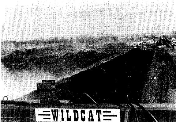
Leaves and grass clippings are windrowed and turned routinely with a Wildcat Compost Turner.
