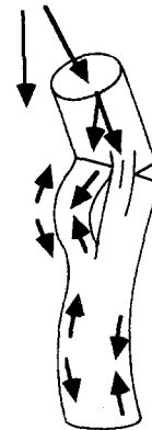
Figure 8. After the face closes pressure in that area increases. Shearing stresses (beyond the scope of this paper) brought on by the increase may induce "barberchair".
