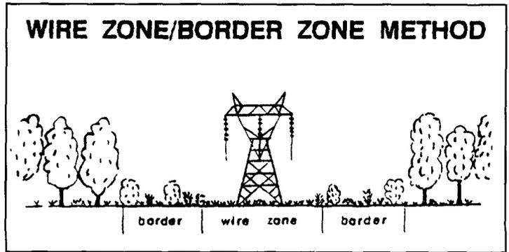
Figure 1. Diagram of a 230-kV line and ROW showing wire zone and border zones. A low shrub-forb-grass cover type is shown on the wire zone; a tall shrub-forb cover type is on the border zones.
