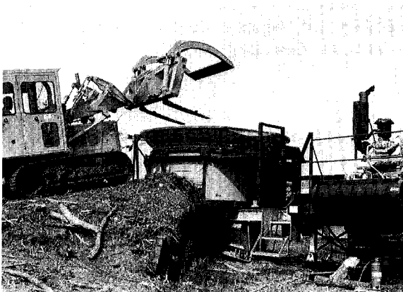
Brush and other woody material under 8 inches in diameter are ground into woodchips using a W.H.O. Tub Grinder.
