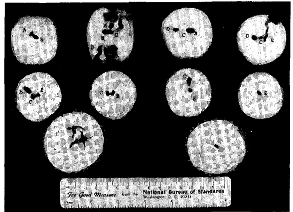
Figure 4. Cross-sections through what must be considered as a strong-compartmentalizing tree, even though borer attacks at chisel-wound site (2nd section from left, upper row) might indicate otherwise. Upper 8 disks, ca. 2 cm thick, sawn sequentially up stem. At time of wounding in October, 1984, tunnels made by 2 borers (A and B) were present in the stem. The borers had exited, but the tunnel of B extended into the next section. Borers C and D attacked at wound site in the autumn of 1983, and were probably P. aureocincta , exiting during autumn of 1985. Borer E entered in summer of 1985 and larva was still present in the tunnel when the tree was felled in the spring of 1986. Lower left section shows typical wood discoloration pattern associated with single borer entrance sites, 2 borers entered at roughly the same level in 2 different years. In all sections, note minimal wood discoloration associated with borer activity. "Flecking" in a portion of the annual ring in bottom right section probably caused by cambium damage upon borer entry, similar to lower left.
