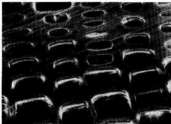
Figure 4. Transverse section of Douglas-fir wood, magnified 675x to show cell cavities and cell walls. (Courtesy of U.S. Forest Products Laboratory.)
