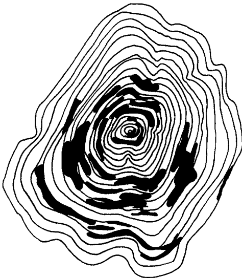
Figure 1. Schematic diagram of carpenter ant nest workings in a cross-section of a trunk. Note that the gnawed portions follow the general pattern of the growth ring.
