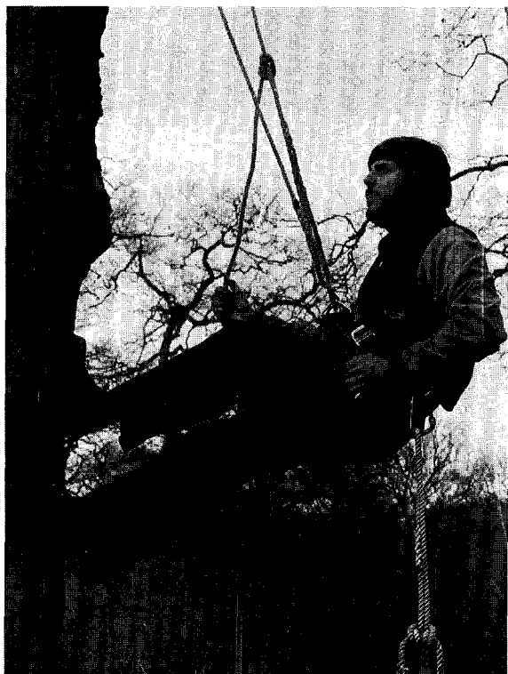
Fig. 6. The prussik knot in action taking the climber's weight, the remainder of the rope being slack and the other end of the loop system parked on the side for ease of illustration. It would normally be parked on the front of the harness.
