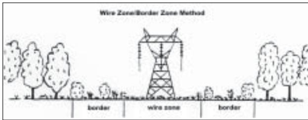
Figure 1. Diagram of a 230-kV electric transmission line, showing wire and border zones. A combination of a low-growing forb–shrub–grass cover type develops in the wire zone, and a tall shrub cover type occurs in the border zone. Adjacent to the border zone is mature forest.
