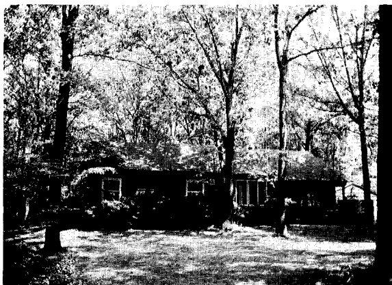
Figure 1. A house well-shaded by deciduous trees that were left standing when the house was built in a woodlot, midday in June.
