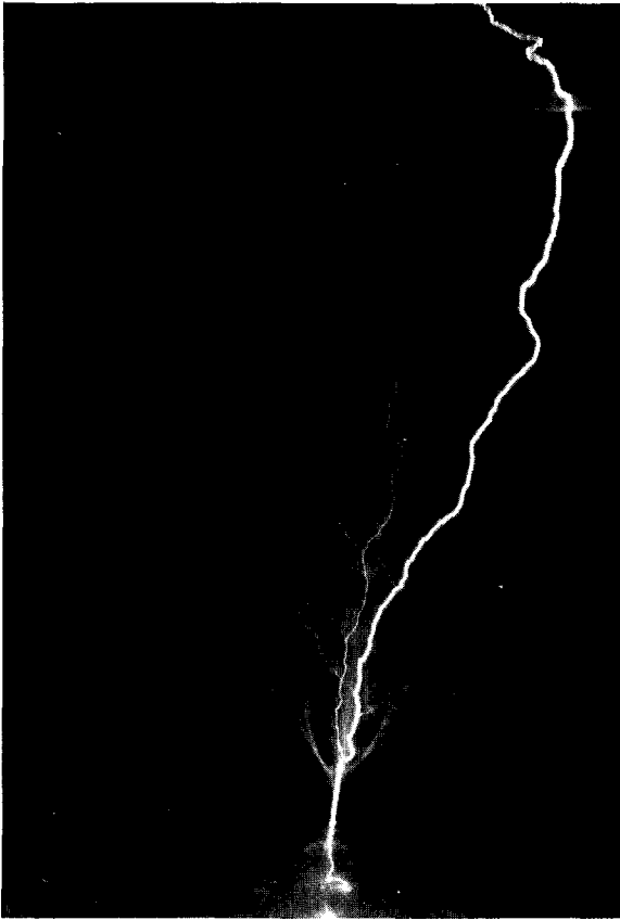
Figure 2. A U+ stroke. The spark starts at the bottom smaller electrode and propagates upward to the larger electrode which acts as the negatively charged cloud. Note branching in direction of propagation.
