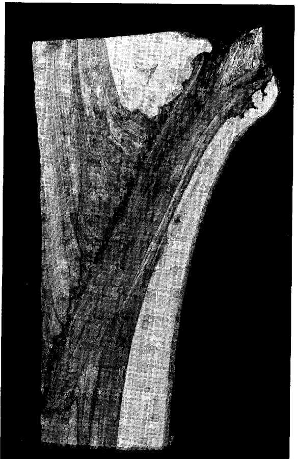
Figure 1.—Dissection of a poorly healed large branch stub on a paper birch. Poorly healed stubs are major external indicators of decay.
