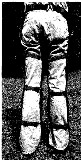
Figure 1. The nylon ballistic leggings earlier required for chain saw operators by EPA. Ruling since rescinded. Front (left) and back (right).
